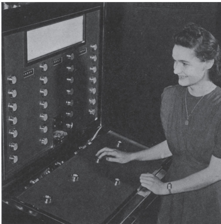
Fig. 2 The Nimatron is a machine which is very skilful at playing the game of Nim (Condon 1942, p 330)
