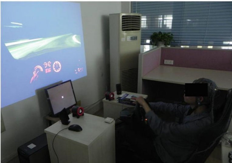
Fig. 1 A typical setup for a study involving the measurements of the mental workload during the drive of a simulated car. The passive BCI return real-time information about the "perceived" mental effort of the subject performing the driving task
