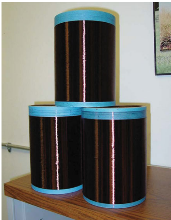
Fig. 1.19 Fiber spools produced from organic-purified hardwood lignin utilizing pilot scale unit with 12-hole spinneret [71]
