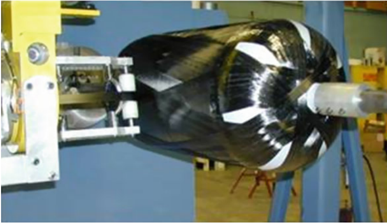
Fig. 7.17 Wet-filament winding process for manufacturing of CNG cylinders
