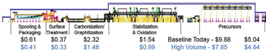
Fig. 8.2 Production cost of PAN-based carbon fibers [1]
