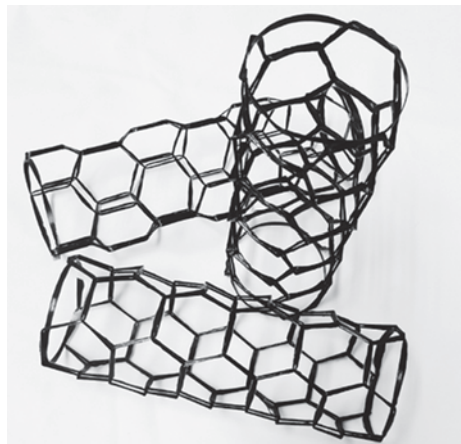
Fig. 7.25 FEM optimized PlanktonTech robot arm ( left ), compared to simulated DLR robot arm ( right )
