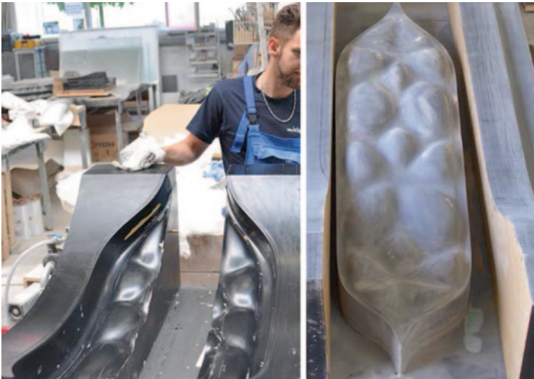
Fig. 6.13 2-part mould ready to laminate the first cells ( left ), 3-part-mould ( right ). (© Fotos: Göran Pohl)
