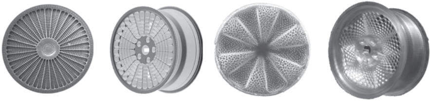
Fig. 11.4 Two Variants of new developments for automotive lightweight wheels. The most important loadcases were tested and revealed very good performances, but an adaptation using evolutionary algorithms has not been executed yet. The left concept has been designed for a realization in anisotropic materials, such as fiber reinforced plastics, the solution on the right is for isotropic materials (e.g. metals)
