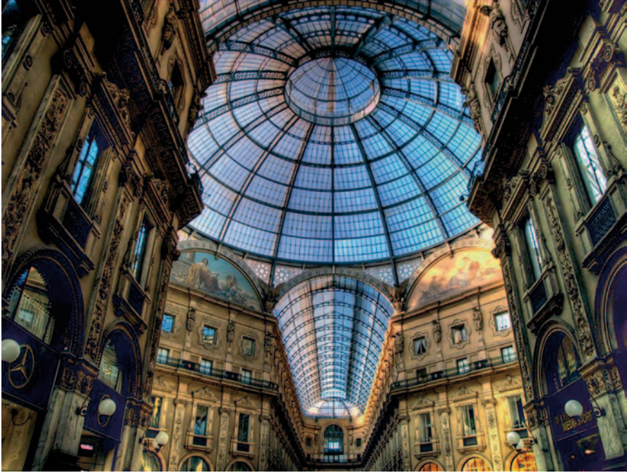
Fig. 5.6 The central dome of Galleria Vittorio Emanuele at Milan, Italy; an example of a glass dome supported by a structure of radial and concentric ribs structurally and functionally similar to that in the valve of the radial centric diatom Arachnoidiscus . http://www.milanexpotours.com/milan-expo-project-2015/numbers/galleria-vittorio-emanuele.html
