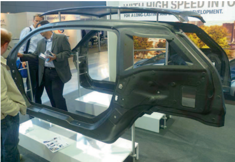
Fig. 7.2 BMW i3 e-car body made from carbon-fiber textiles
