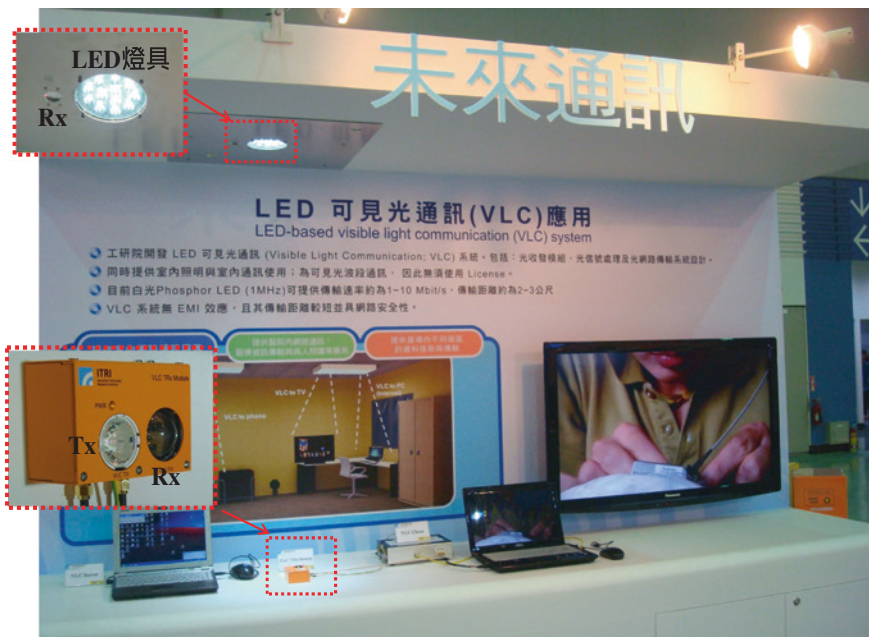
Fig. 4.14 Real-time bi-directional LED VLC system using IR uplink
