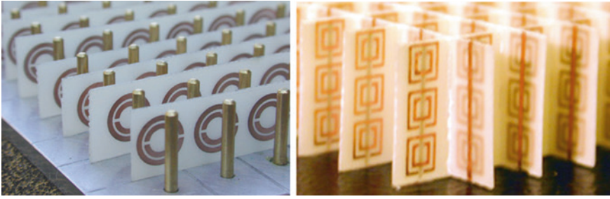
Fig. 2.2 Two typical metamaterials consisting of metallic structures, both have negative refractive index in a certain frequency range. The metallic wires or rods provide the negative permittivity and the split-ring resonators provide the negative permeability. (Images: Physics Today, May 2000, 17; Science Vol. 292: 77, 2001)
