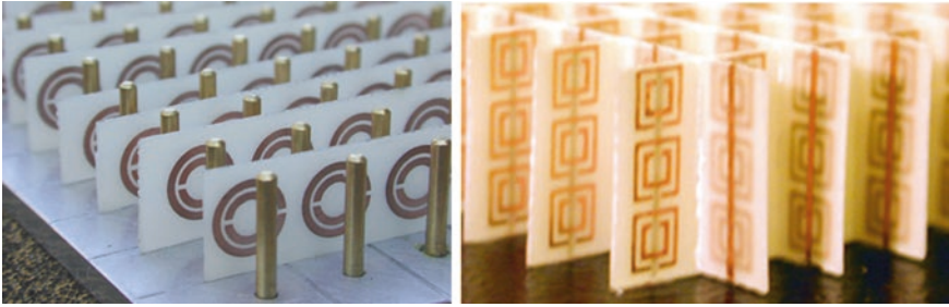
Fig. 2.2 Two typical metamaterials consisting of metallic structures, both have negative refractive index in a certain frequency range. The metallic wires or rods provide the negative permittivity and the split-ring resonators provide the negative permeability. (Images: Physics Today, May 2000, 17; Science Vol. 292: 77, 2001)
