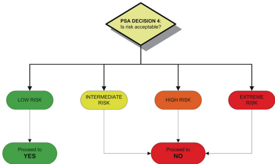
Fig. 11 Decision (4) on whether or not the risk posed by the ballast water intended for discharge is acceptable (This figure can be downloaded from http://extras.springer.com/ )
