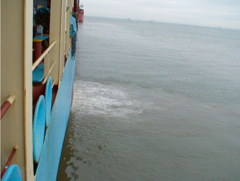
Fig. 7 Discharge of ballast water below the water level from a container vessel
