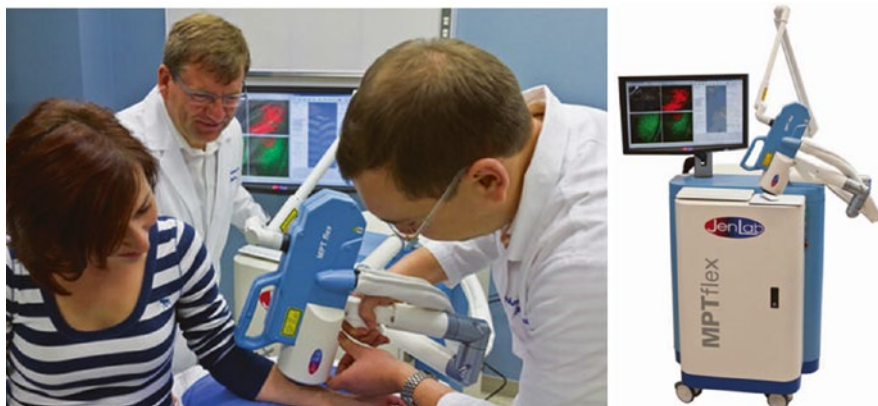
Fig. 16.9 Clinical multiphoton microscope that can be equipped with TCSCP FLIM (From König (2012)). [Copyright permission being sought]
