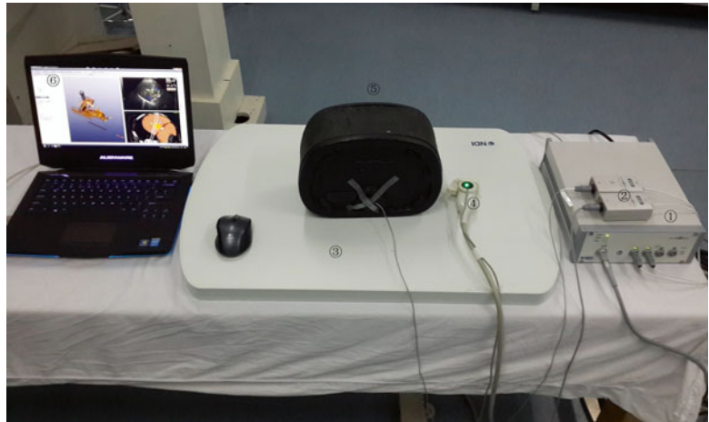
Fig. 27.1 Physical setup and components of three-dimensional (3D) visualization preoperative treatment planning system. Legend: ① a control unit of the electromagnetic tracking system ② two sensor interface devices of the electromagnetic tracking system ③ a field generator of the electromagnetic tracking system ④ tracked ultrasound probe ⑤ a simulation model ⑥ screen
