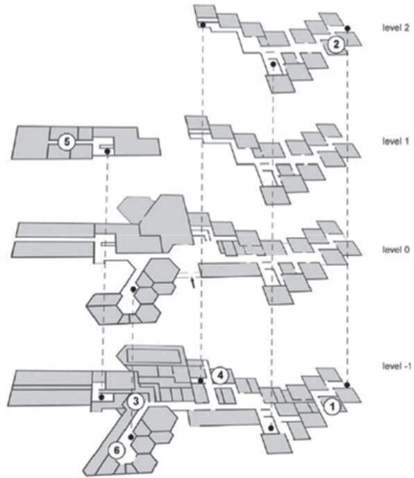
Fig. 5 Stacked, diagrammatic floorplan of the conference centre site used by Hölscher et al. for their study of multi-level wayfinding. Note the disparities between different floors [43]
