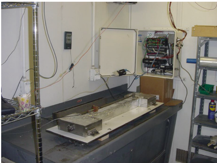
Fig. D.25 Autogenous deformation measurement in sealed samples
