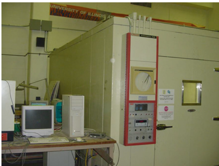
Fig. D.23 Environmental chamber and relative humidity system
