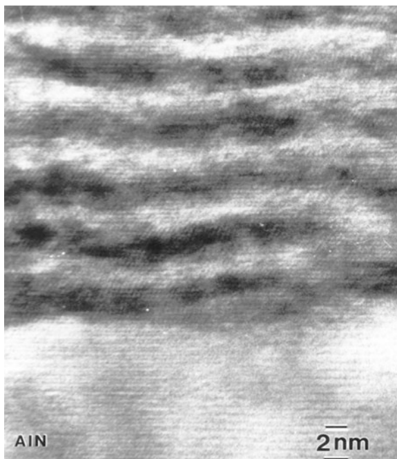
Fig. 3 A single crystalline ZrN/AlN multilayer grown on a heteroepitaxial AlN buffer layer. The composition modulation wavelength is 3.4 nm. The dark and bright layers are respectively ZrN and AlN (after Meng and Voyiadjis [3])
