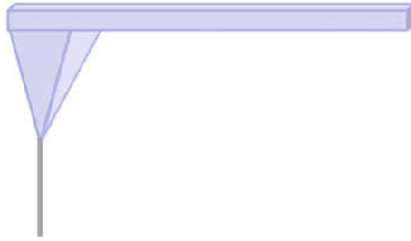
Fig. 10 The atomic force microscope (AFM) probe with the high aspect-ratio carbon nanotube tip (the orientation of the tip attachment is not completely vertical due to the orientation of the faces of the pyramidal tip)
