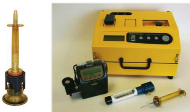
Fig. 6.7 The ADS surface sampling SPME interface ( left ) and the SPS-3 field-portable vapor and liquid sample preparation station ( right )
