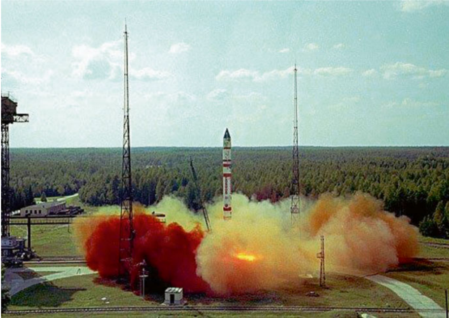
Fig. 18.3 Dense red clouds of highly toxic nitrogen oxides and heptile around the space rocket on launch
