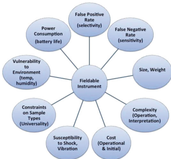
Fig. 6.5 Tradeoffs in miniaturizing mass spectrometers
