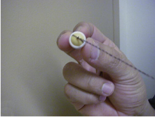
Fig. 4.3 A string-capsule endoscope. Reprint with permission from Gastrointest Endosc [56]
