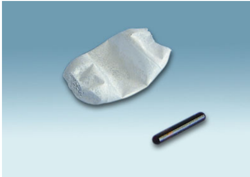
Fig. 3.45 Disintegrated capsule remnants: empty shell and RFID tag
