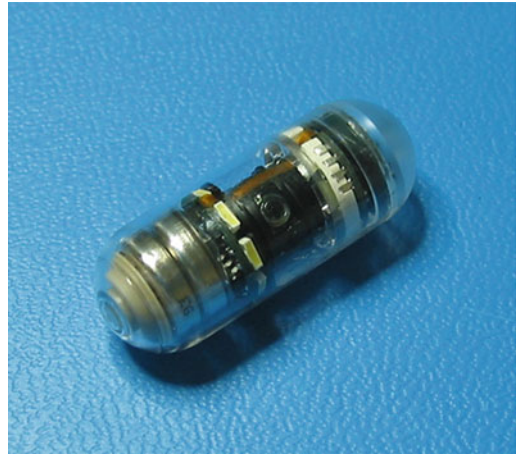
Fig. 2.34 The CapsoCam SV1. Reprint with permission from Friedrich et al. [132]
