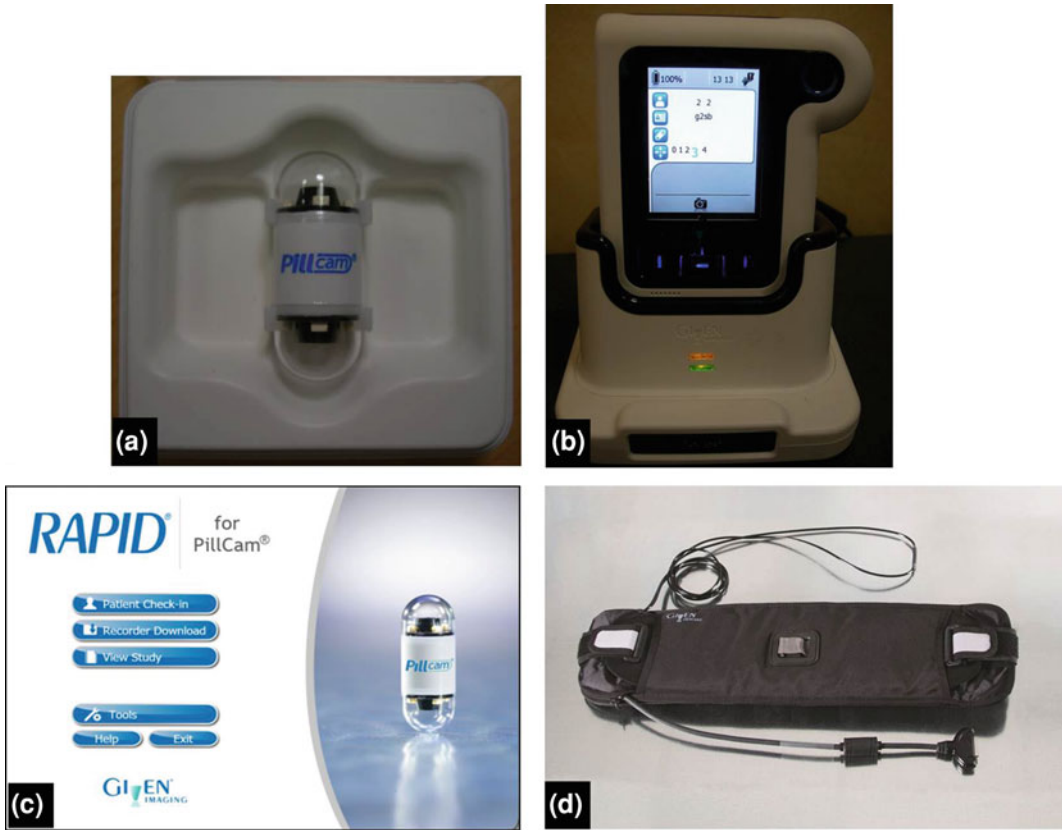
Fig. 5.1 The new generation of colon capsule endoscopy system. a The second generation colon capsule (PillCam colon 2, given Imaging, Israel) is 11.6 x 31.5 mm in size and has 2 optical domes with an angle of view of 172° for each imager. The data recorder (b) besides storing the images transmitted from the capsule also (i) controls the capsule image rate in real
