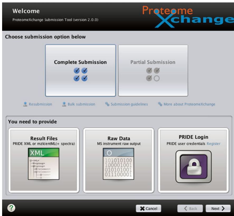
Fig. 4.6 PX submission tool's main interface. First, user should select submission option. For a complete submission is mandatory to enclose a result file formatted as PRIDE XML or mzIdentML plus the unprocessed raw data
