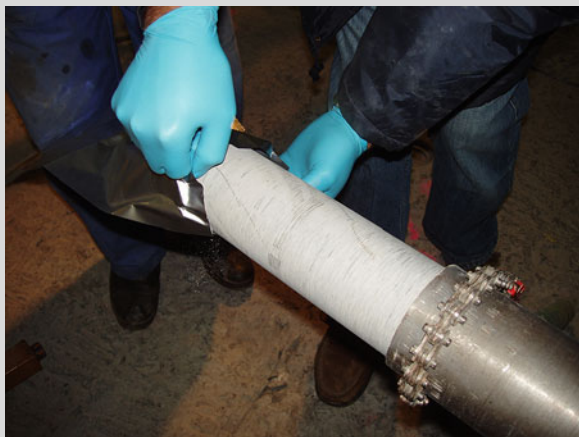
Box Fig. 17.1 Extraction of a core from a geological clay formation (Photograph: Laurent Urios)
