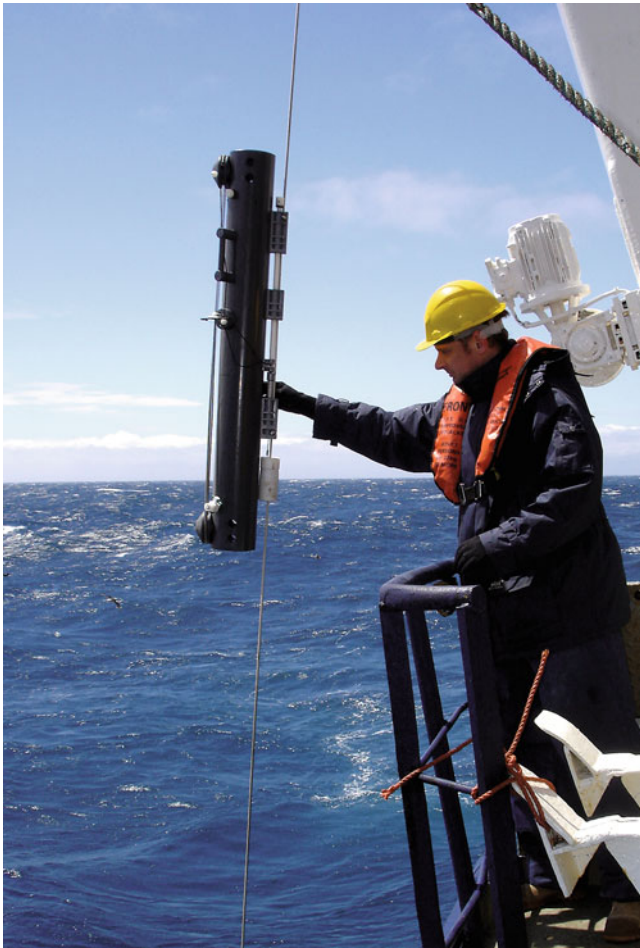
Fig. 17.3 Go-Flo on the line ready to be dropped into the water. The Go-Flo has the advantage of passing through the sea surface microlayer closed, and thereby avoids its inner surface being coating with a surface film rich in contaminants (Photograph: Patrick Raimbault)
