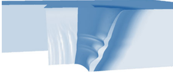
Fig. 6 Ablation simulation for laser cutting
