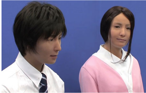
Fig. 1 The very life-like android robot Actroid in the male and female version. The appearance of this robot is so close to a real human that, on a picture, it is very difficult to distinguish it from a real human. This experiment used the Actroid-F, the female version of the android robot
