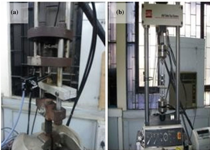
Fig. 2 Setup for small punch testing, a fixture for small punch testing and b installation of fixture on MTS 858 table top machine
