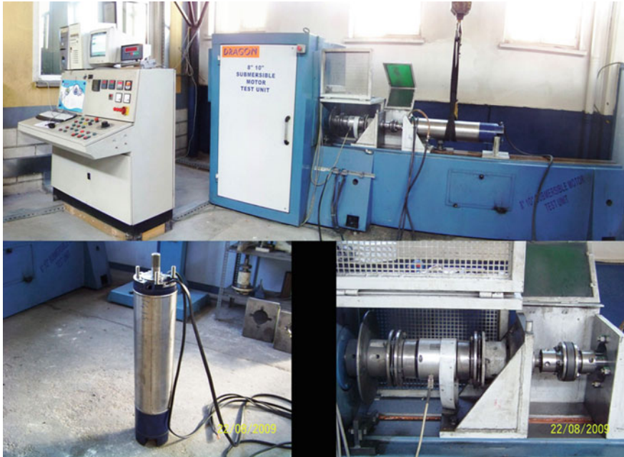
Fig. 6 Photographs of experimental system, SIMS and torque–speed sensor
