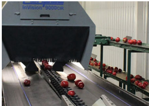
Fig. 1 Example of the commercial machine used to capture images and extract features for the training of classifiers
