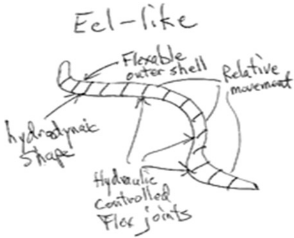
Fig. 4 Concept based directly on a biological system, instead of drawing an analogy [5]
