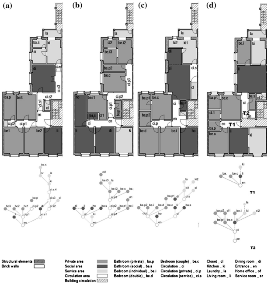
Fig. 4 a Original dwelling: rehabilitated dwellings, floor plan and graph, according to the three strategies; b 1st strategy; c 2nd strategy; d 3rd strategy
