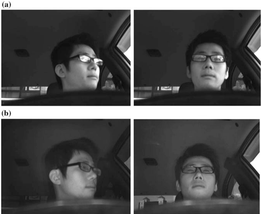
Fig. 6.4 Reflected sunlight is dealt with by an NIR illuminator with a narrow bandpass filter (a NIR illuminator only, b NIR illuminator with bandpass filter) in [37]
