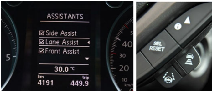
Fig. 9.27 Implementation of the HMI Controller (VW and Honda)
