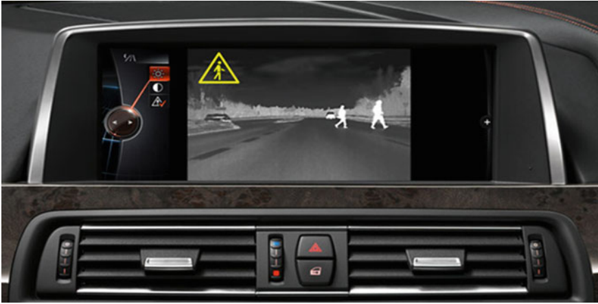
Fig. 5.30 Successful detections via IR image [37]
