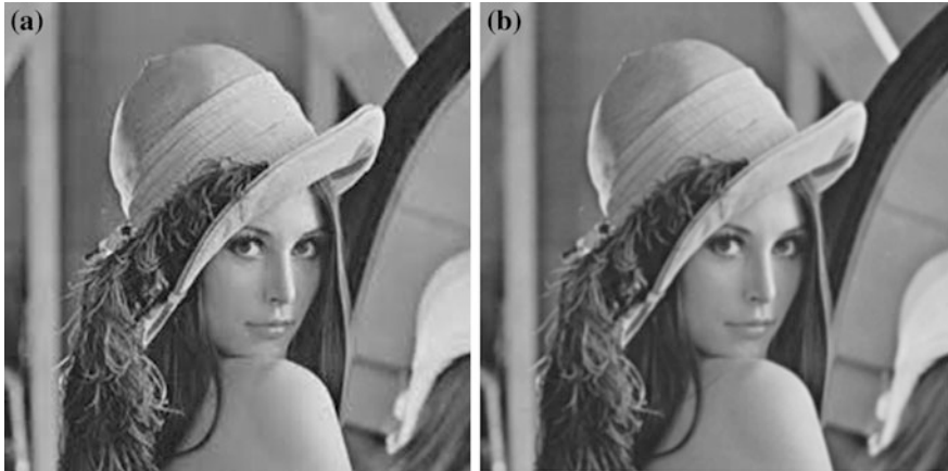
Fig. 4.8 Result of low pass filtering a Original image. b Low pass filtered image
