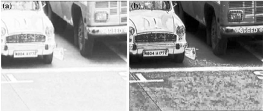
Fig. 4.20 Low contrast image and contrast stretched image a Low contrast image b Contrast stretched image
