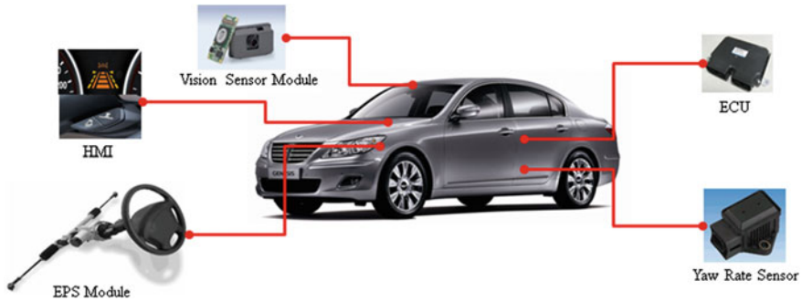
Fig. 9.22 Components of the LKAS
