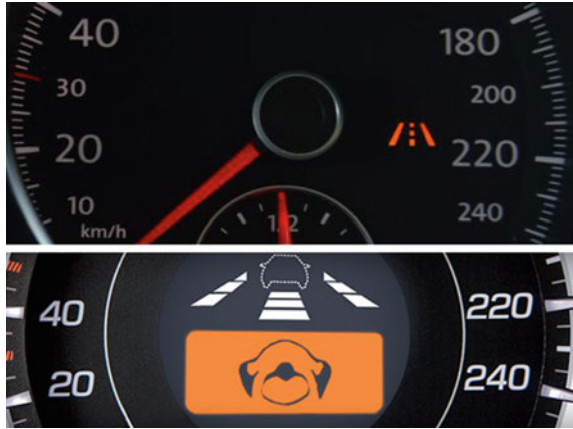
Fig. 9.26 Implementation of the HMI Indicator (VW and Honda)
