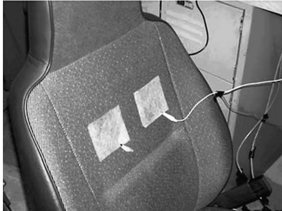
Fig. 6.7 ECG measurements on driver's seatback from [55]
