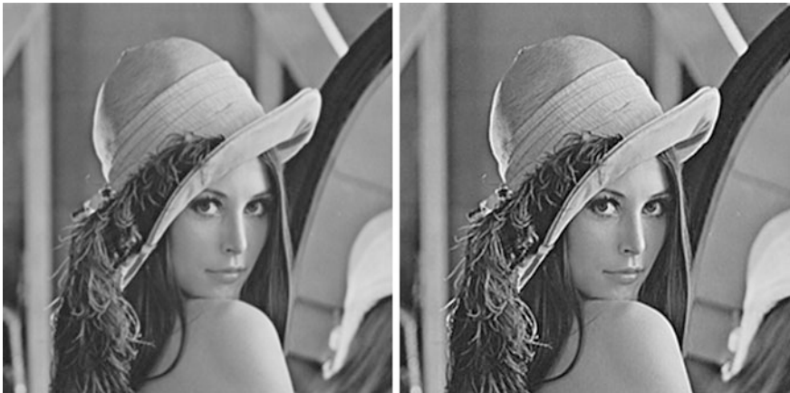
Fig. 4.11 Example of unsharp masking
