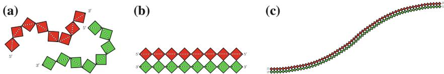
**Fig. 7.2** Single and double stranded mDNA: **a** single stranded mDNA, **b** double stranded mDNA, **c** double stranded mDNA has a longer persistence length
