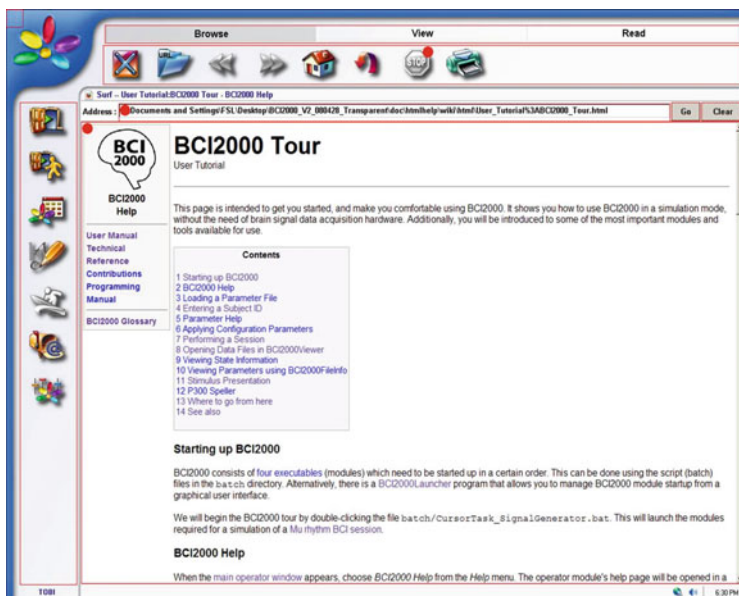
Fig. 2.3 Connection of the commercially available software QualiWorld (QualiLife SA, Paradiso, Switzerland) and the P300 BCI. Instead of letters, red dots are being flashed, indicating the link on the screen to be chosen
