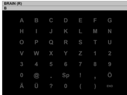
Fig. 2.1 Example of a P300 Speller matrix. Letters of the alphabet are arranged in rows and columns as are numbers and additional punctuation marks
