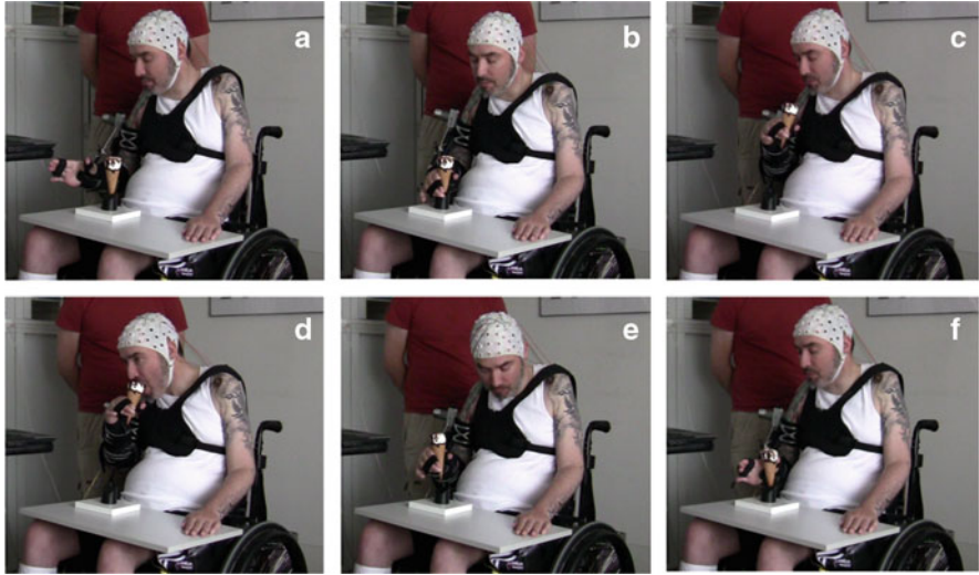
Fig. 2.9 Sequence of pictures showing the eating of an ice cone. The user starts in the hand control mode, lifts his left shoulder to open the right hand for grasping the ice cone (a). After successfully grasping the ice cone (b), the user emits a BCI command to switch from hand control to elbow control and lifts his shoulder to flex his elbow (c). Now, the user licks the ice (d). Finally, the user lowers his left shoulder to extend the elbow (e), he puts the cone in its original place and switches back to hand mode to release the cone (f)
