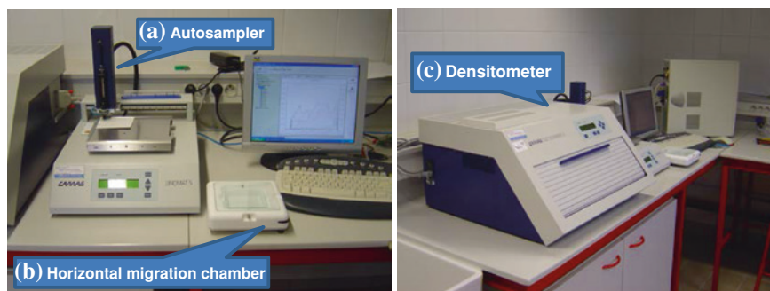
Fig. 16 HPTLC basic instruments from CAMAG. a Autosampler: The sample is deposited onto the HPTLC plate using a syringe. The sample is band wide sprayed (suitable for automatic detection). The spraying gas is generally nitrogen. The number of bands and their width as well as the sprayed volume and deposition speed are programmed depending on the number of deposited samples, nature of solvent (volatility), and the concentration of analytes, respectively. b Horizontal migration chamber: separations can be carried out from two sides in unsaturated, saturated, and sandwich configuration but single-sided developments are also possible. c UV–Visible scanner for densitometric evaluation of TLC/HPTLC chromatograms. The scanner can work either in absorbance, reflectance, or fluorescence mode
