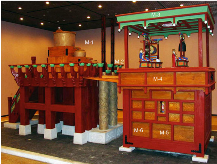
Fig. 6 Reinstated replica of the Striking Palace Clepsydra (frontal view). The labels M-x are the same as in Fig. 5. The whole installation measures approximately 6 m in width, 2 m in depth, and 5.7 m in height. (Photo by Nam 2006)
