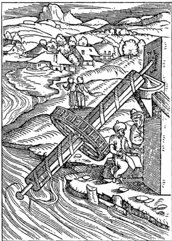
Fig. 25 Drawing of an Archimedes screw pump in Barbaro's edition in 1584 on page 463
