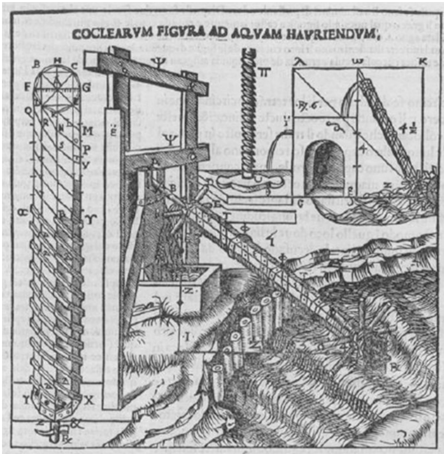
Fig. 23 Drawing of an Archimedes screw pump in Cesariano's edition in 1521 on page CLXXI v
