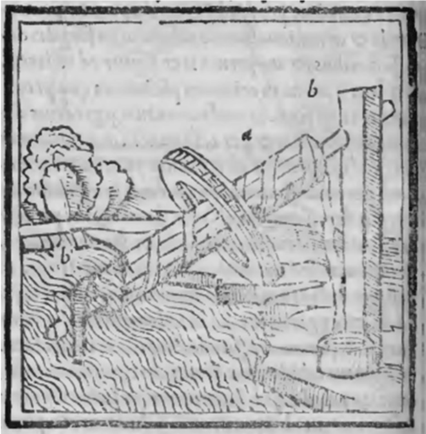
Fig. 22 Drawing of an Archimedes screw pump in Fra Giocondo's edition in 1513 on page 172 v
