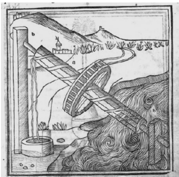
Fig. 24 Drawing of an Archimedes screw pump in Durantino's edition in 1524 on page 102 r
