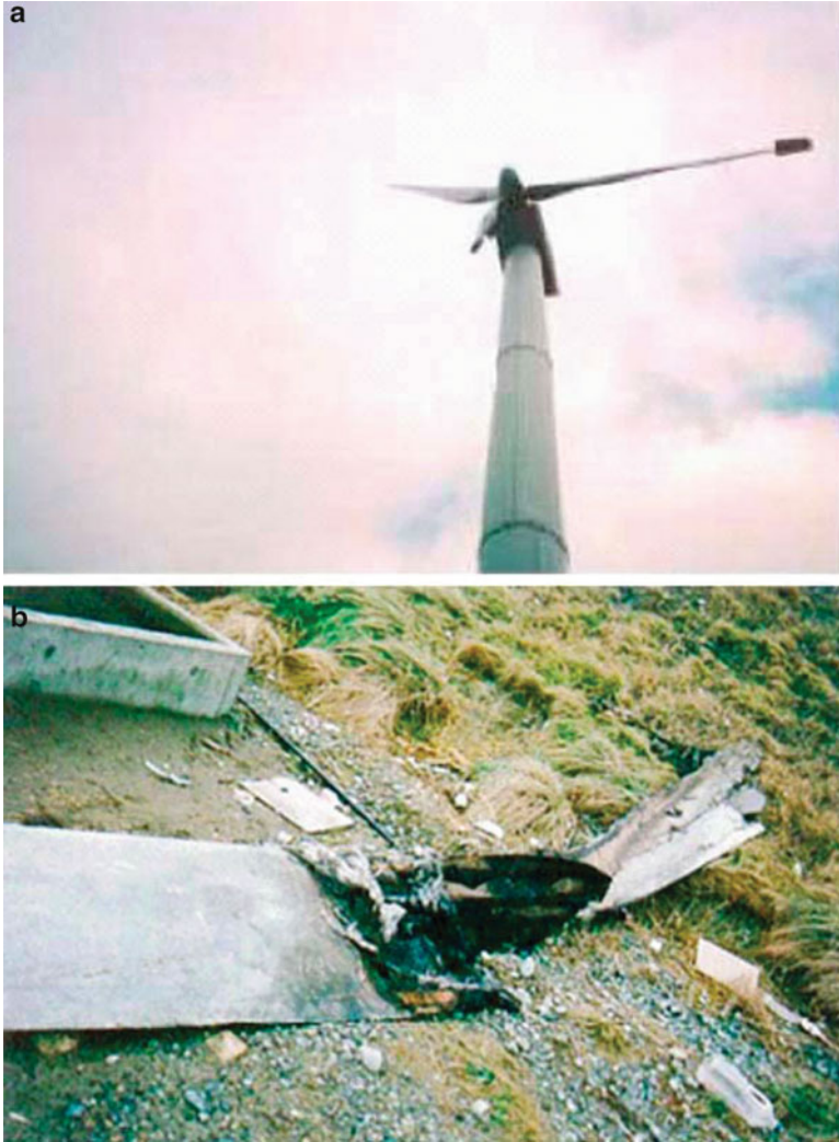
Fig. 15.18 Damage caused by lightning flash in wind turbine blade (adapted from [10])
