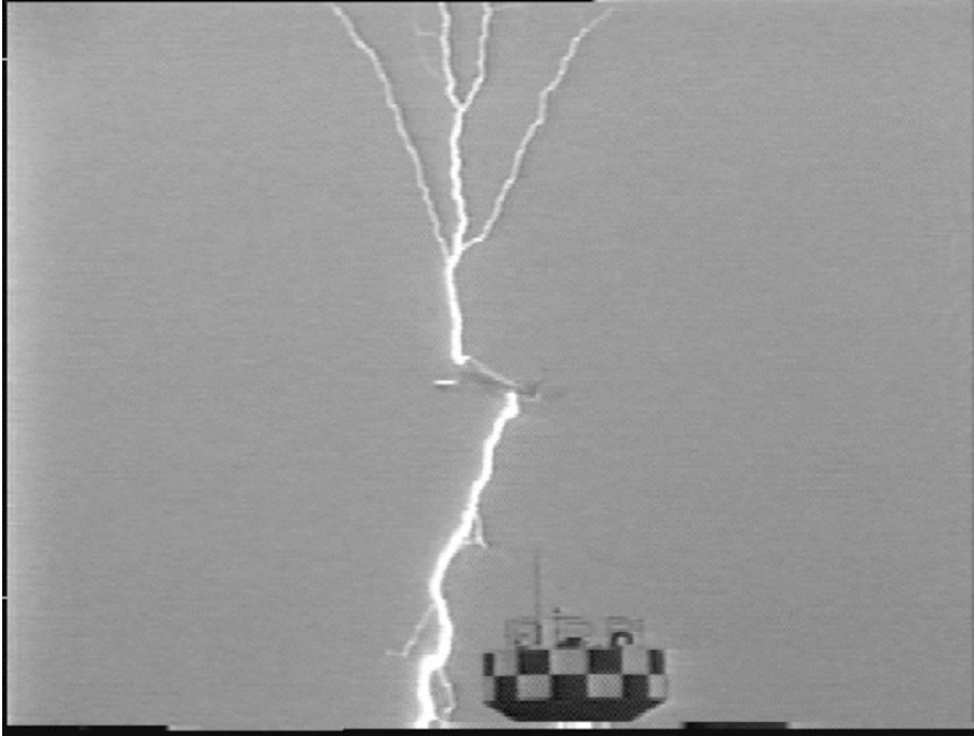
Fig. 15.11 Video frame of a lightning strike to an aircraft on takeoff from Kamatzu Air Force Base on coast of Sea of Japan during winter. Note that the branches of the upper part of the channel are directed upward, whereas the branches on the lower part of the channel are directed downward. This shows that a bidirectional leader started from the plane with one part propagating upward and the other downward (Courtesy Prof. Z.I. Kawasaki)
