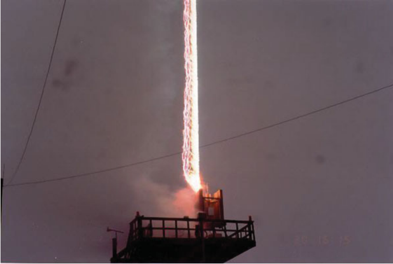
Fig. 20.7 Different strokes of triggered lightning flash separated in space due to movement of channel in wind during interstroke time interval (Courtesy Prof. V. Rakov, University of Florida at Gainesville, Florida, USA)
