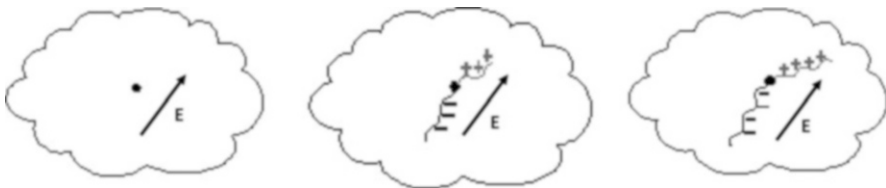
Fig. 7.3 Bidirectional propagation of a leader. Initiation of a leader inside a cloud gives rise to two leader branches, one charged positively and the other negatively, and moving in opposite directions along the field lines of the background electric field. The net charge on the leader channel is zero. In other words, the positively charged leader branch provides the negative charge for the development of the negatively charged branch, and vice versa (Figure created by author)
