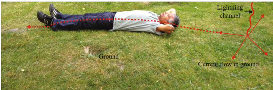
Fig. 16.8 A person lying down on the ground can be exposed to ground currents that pass through the heart. In this case, since different parts of the ground are at different potentials, a current could enter the body from the person's head and pass to the ground from different parts of the body that are in contact with ground. In this situation, the current may flow both through the brain and the heart and could inflict severe injuries (Figure created by author)
