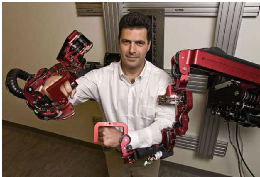
Fig. 15.1 The upper limb exoskeleton EXO-UL7 with seven DOFs, supporting 99% of the range of motion required to perform daily activities
