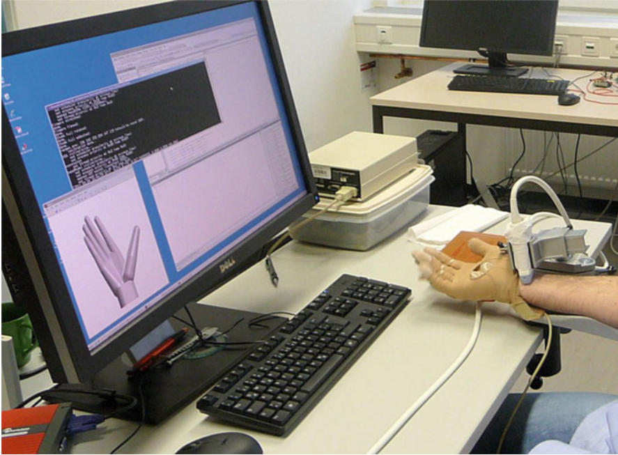
Fig. 2.7 The experimental setup used in [5, 8] to record US images and metacarpophalangeal angles. A 3D hand model would teach the subject the motion to imitate; the ultrasound probe was held against the subject’s wrist using a vise; and a dataglove was used to collect the MCP joint angles
