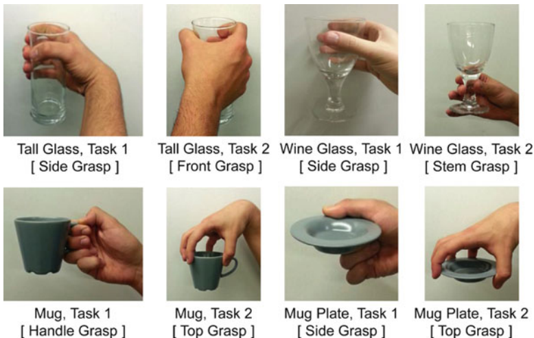
Fig. 1.2 Tasks executed for the second type of experiments. The tall glass tasks were: task 1, side grasp (to drink from it) and task 2, front grasp (to transpose it). The wine glass tasks were: task 1, side grasp (to drink from it) and task 2, stem grasp (to drink from it). The mug tasks were: task 1, handle grasp (to drink from it) and task 2, top grasp (to transpose it). Finally the mug plate tasks were: task 1, side grasp (to lift and hold it) and task 2, top grasp (to transpose it)
