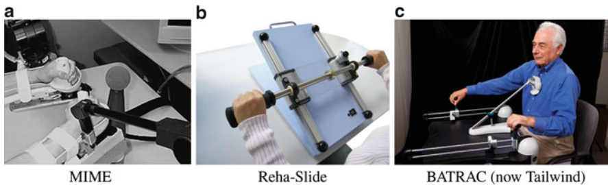
Fig. 14.5 Several of the devices that have been used for bimanual rehabilitation. The general idea of bimanual rehabilitation is that an individual assists his own paretic arm with his sound arm through an external physical coupling (Subfigure (a) reproduced from [48] under the Creative Commons Attribution License. Subfigures (b) and (c) reproduced with permission)
