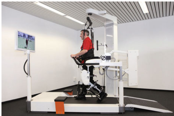
Fig. 14.6 The Lokomat® is a gait-assistive device with a built-in body weight support system (Picture: Hocoma, Switzerland)
