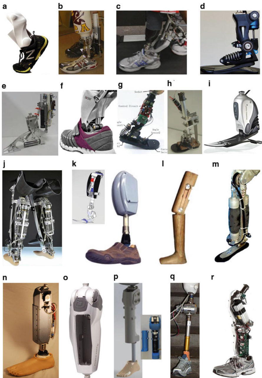
Fig. 5.8 Active prosthetics for the ankle (a–j) the knee (k–q) and for both joints (r). For a more detailed description see Table 5.3 for the ankle and Table 5.4 for the knee joints (Appendix)
