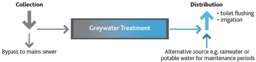
Fig. 27.5 Greywater reuse system. Source City of Melbourne (2011)
