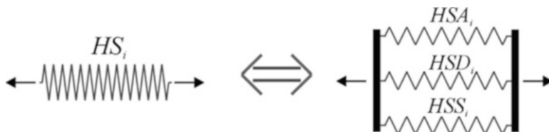
Fig. 24.11 Each horizontal spring consists of three components to account for aggregate interlock (HSA), the dowel effect (HSD), and the shear/horizontal reinforcement (HSS) mechanisms
