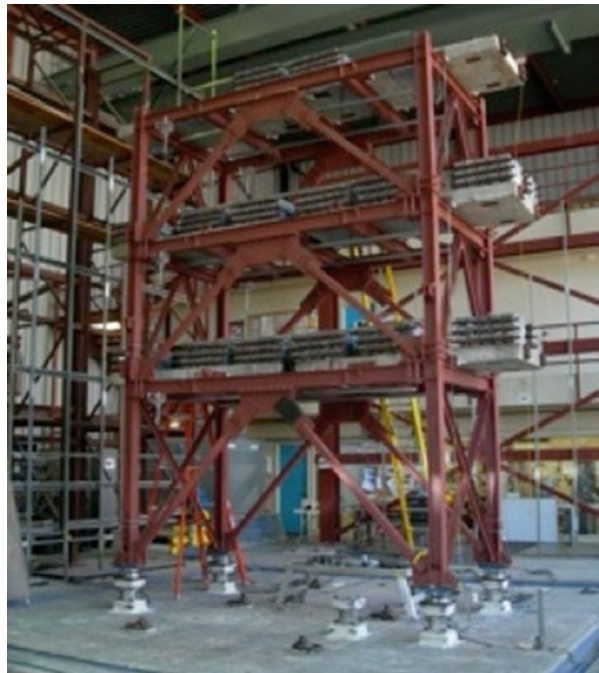
Fig. 2.4 Test of isolated 3-story building
