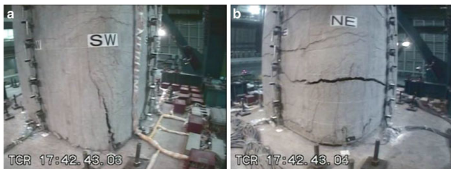
Fig. 13.6 Damage of C1-6 column during 2–125 % (3) excitation (a) SW corner (b) NE corner
