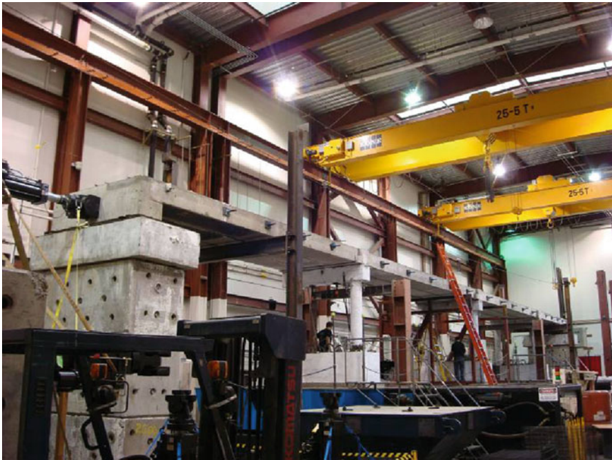
Fig. 5.3 Four-span bridge model
