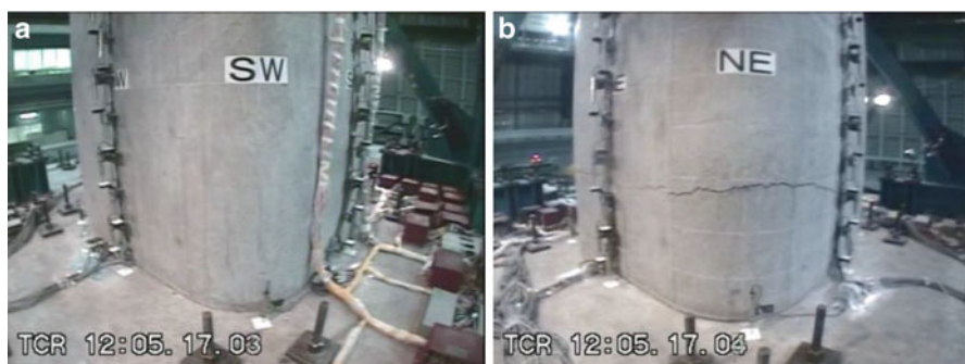
Fig. 13.5 Damage of C1-6 column during 2–100 % excitation (a) SW corner (b) NE corner
