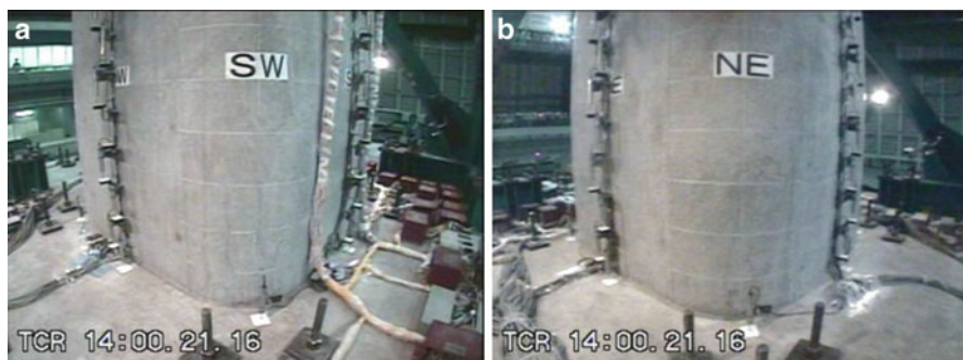
Fig. 13.4 Damage of C1-6 column during 1–100 % (1) excitation (a) SW corner (b) NE corner
