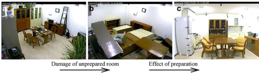
Fig. 16.15 Test result of residential room: (a) initial condition of unprepared room at 0 s, (b) damage of unprepared room at 130 s, (c) damage of prepared room at 130 s
