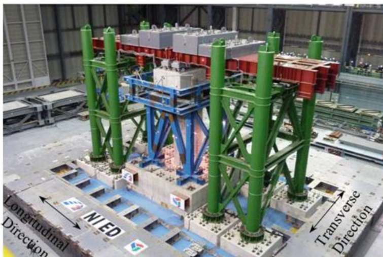
Fig. 13.2 Experiment set-up using the E-Defense shake-table
