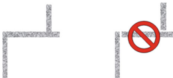
Fig. 11.7 The whole flange width of a flanged section must be considered (T, L, C, or other cross sectional shapes)
