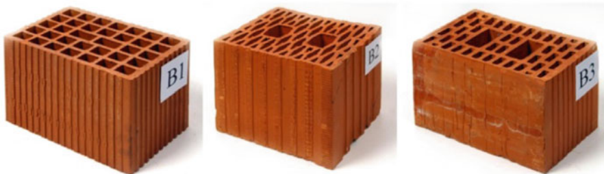
Fig. 25.6 Typical hollow clay blocks tested in the experimental campaign (After Tomažević and Weiss 2012)
