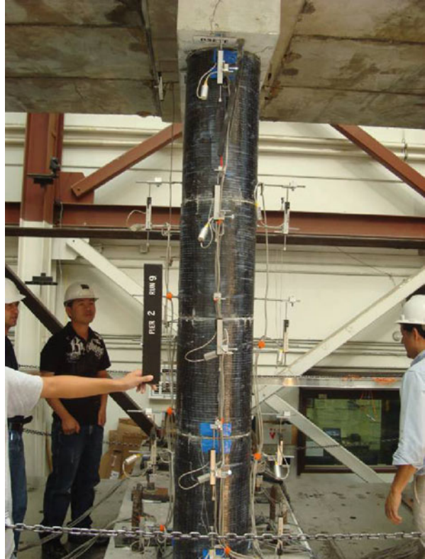
Fig. 5.13 FRP-wrapped, segmental bent after shake table test
