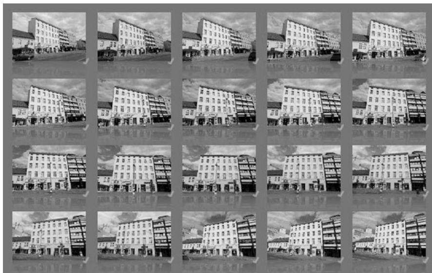
Fig. 8.17 Always try to keep the whole façade in the view port of the camera
