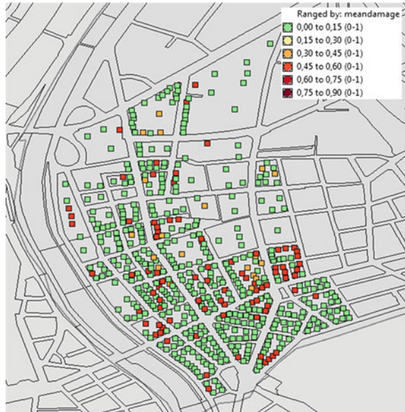
Fig. 8.25 Building damage for the “method testing” earthquake
