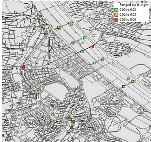
Fig. 8.30 Road bridge damage for the “Neulengbach” earthquake
