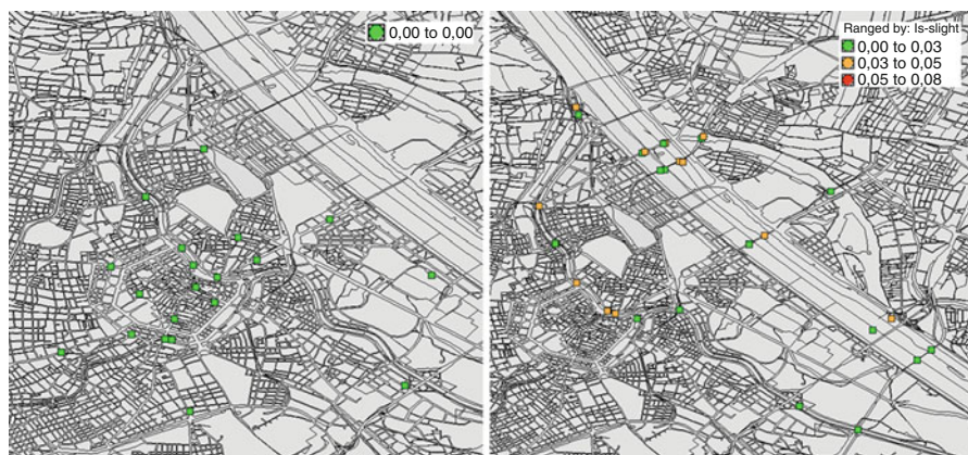
Fig. 8.29 Railway tunnel ( left ) and bridge ( right ) damage for the “Neulengbach” earthquake
