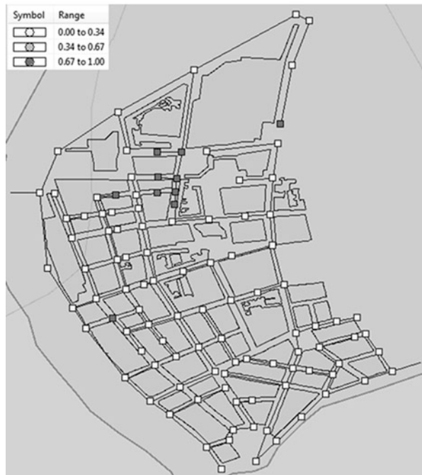
Fig. 8.47 Damage level on the electric power network for the selected scenario
