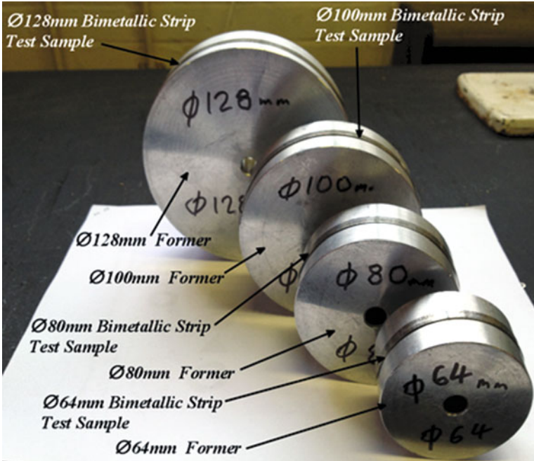
Fig. 5 Test samples checking for roundness and size
