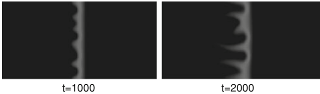
Fig. 6 Concentration iso-surfaces for \alpha = 0.3 , R_b = -1 , R_c = 5 (unstable trailing front, stable leading front)
