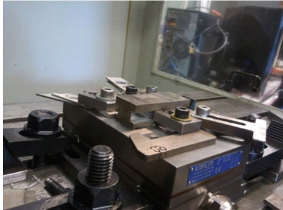
Fig. 1 Workpiece clamped onto dynamometer
