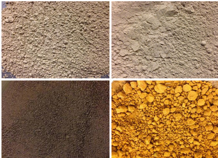
Fig. 11.1 Pictures of example phosphorus sorbing materials ( PSMs ) that are industrial by-products. From top left moving clockwise: fly ash, gypsum, acid mine drainage treatment residuals ( AMDRs ), and drinking water treatment residuals ( WTRs )
