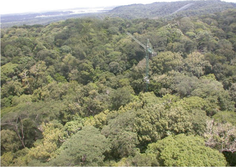
Fig. 22.1 Crane in Area Protegida de San Lorenzo, Colon, Caribbean coast. This crane has access to 0.9 ha. Canopy height is 35–45 m (Picture: IBISCA-PANAMA project)
