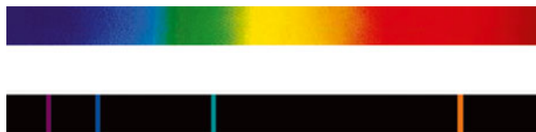
Fig. 15.1 Continuous spectra of solids ( above ) and line spectra ( below ) for hydrogen
