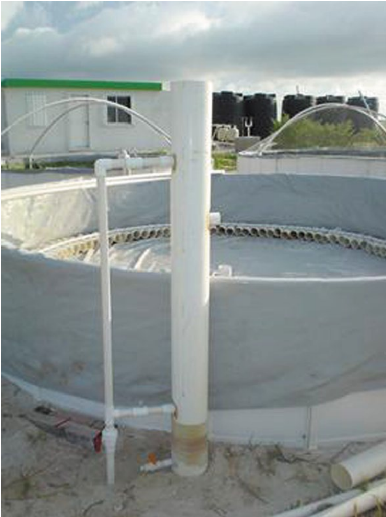
Fig. 20.6 Protein skimmer that eliminates organic material of recirculatory seawater system in Octopus maya culture. (Rosas et al. 2014)
