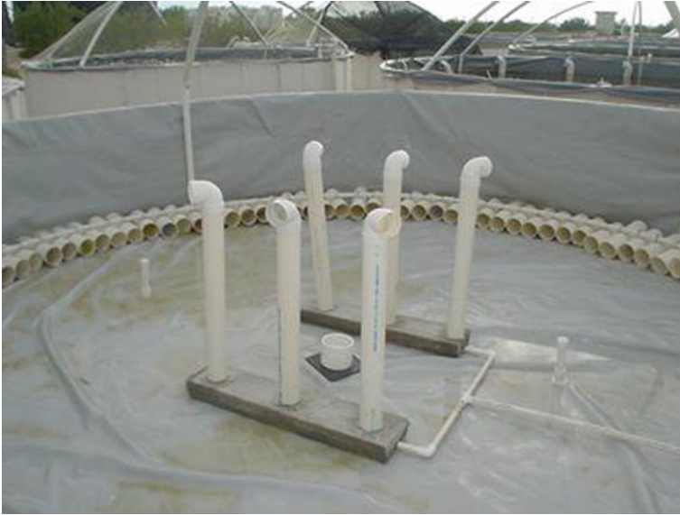
Fig. 20.5 Aeration system for Octopus maya on-growing ponds based on airlift pumps. (Rosas et al. 2014)
