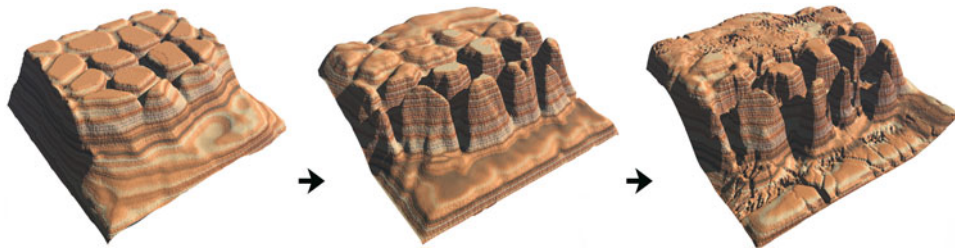
Fig. 6.5 Sequence of block diagrams illustrating the development of monoliths on thick and massive conglomerate successions affected by widely spaced orthogonal fractures (Illustration produced by Santiago Alberto-Moralejo)
