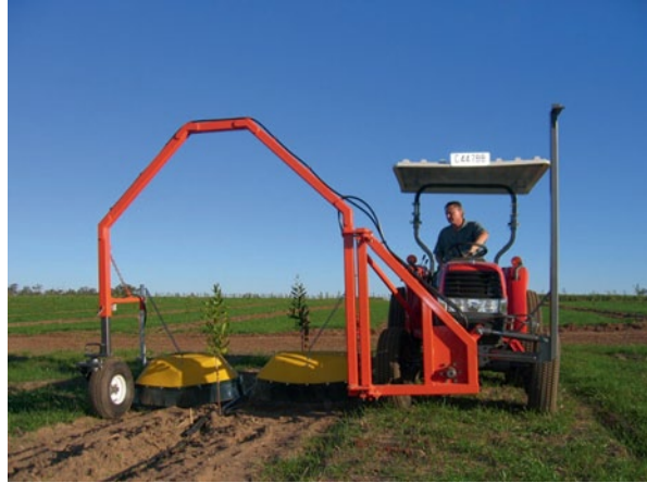
Fig. 8.26 Herbicide sprayer used on newly planted trees. Trees passed between the two shielded hoods. This machine is used until the trees are 2–3 years old. (©Searle)
