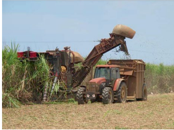
Fig. 8.3 Mechanical harvesting of sugarcane. (©Diczbalis)
