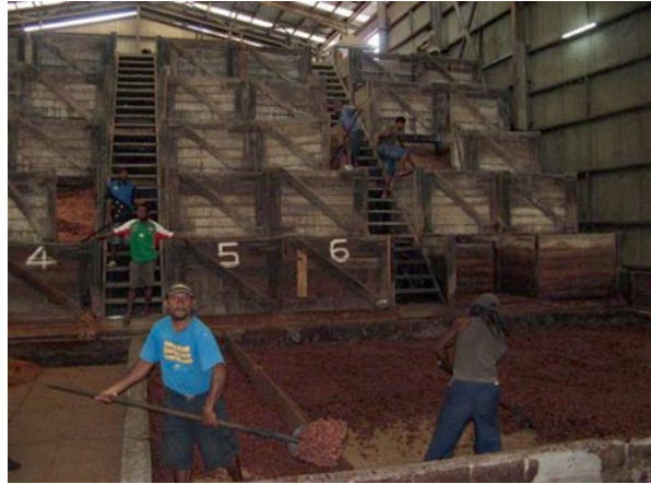
Fig. 8.18 Large and efficient cascading box fermentation facility in Papua New Guinea. (©Lambert)
