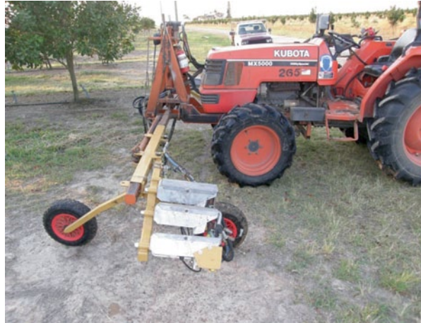
Fig. 8.27 Herbicide sprayer used on older trees. A sensor detects the presence of green weeds and applies herbicide directly to them. (©Searle)
