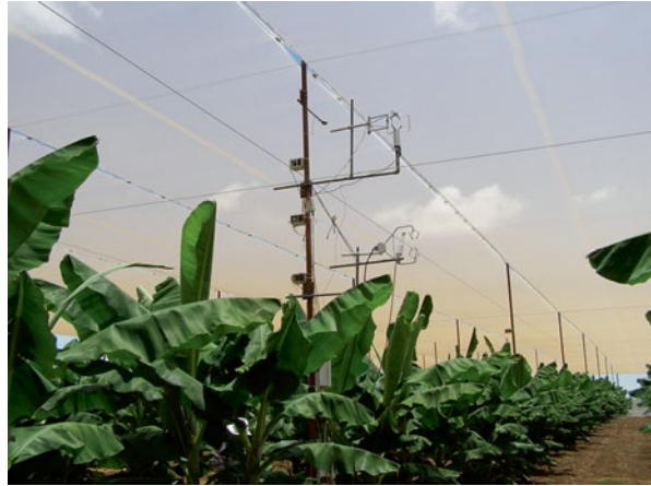
Fig. 10.14 Two eddy covariance systems installed in a large banana screenhouse, located at the Western Galilee of northern Israel. The systems measure whole canopy turbulent fluxes of water vapor, heat and \text{CO}_2 . Their deployment above the canopy does not interfere with the crop. (Source: Tanny 2007, private collection)
