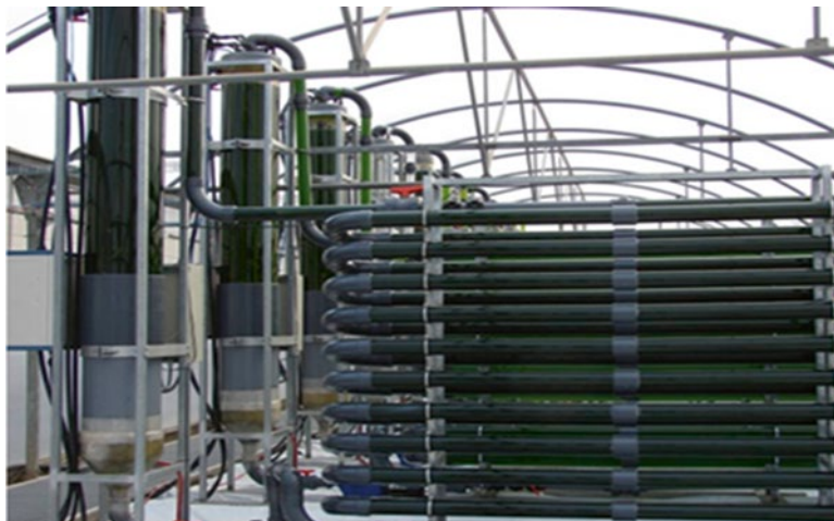
Fig. 13.8. Photograph of an industrial size fence configuration tubular photobioreactor 30 m 3 plant for the production of lutein from Scenedesmus almeriensis Almería. Fundación CAJAMAR (With permission of Fundación CAJAMAR, Almería, SPAIN).
