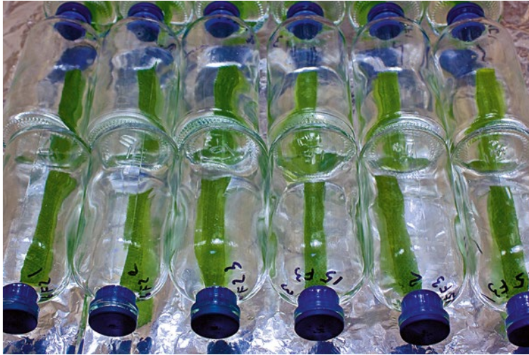
Fig. 14.1. The entrapment of Chlamydomonas reinhardtii cells in \text{Ca}^{2+} -alginate films is a convenient way for screening \text{H}_2 photoproduction activities in different mutants.
