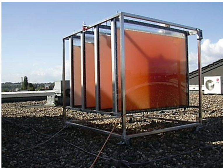
Fig. 11.6. Modular arrangement of flat panel reactor (112 L) operated at RWTH, Aachen (Reproduced with permission from Gebicki et al. 2010).
