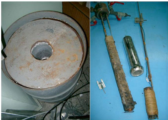
Fig. 15.1 Early hand-made devices at SCUH. Left panel: A magnetic shield for the characterization of ceramic SQUIDs. The walls were made out of hundreds of metal sheets accommodated in an oil can, surrounding a glass dewar which was inserted into the hole. Notice the “brand name” written on top: “Tropical SQUIDs, Inc.” Right panel: assorted parts to study transport properties of superconductors at low magnetic fields (the long solenoid allowed the temperature to be controlled by moving the sample along its axis, without losing the uniformity of the magnetic field)
