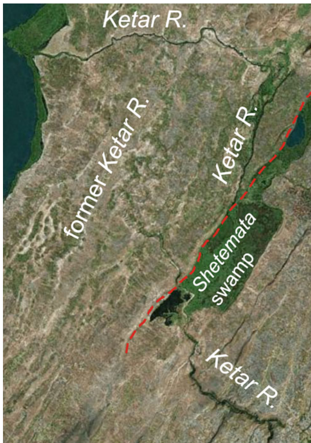
Fig. 4.4 The old channel of the Ketar River in the plain of Ogolcho ( 08^{\circ} 00' 00''\text{N} – 38^{\circ} 59' 00''\text{E} ). The river abandoned the old channel and moved into its present position in connection with the movement of the normal fault indicated by the dashed red line (modified from Corti and Manetti 2012)
