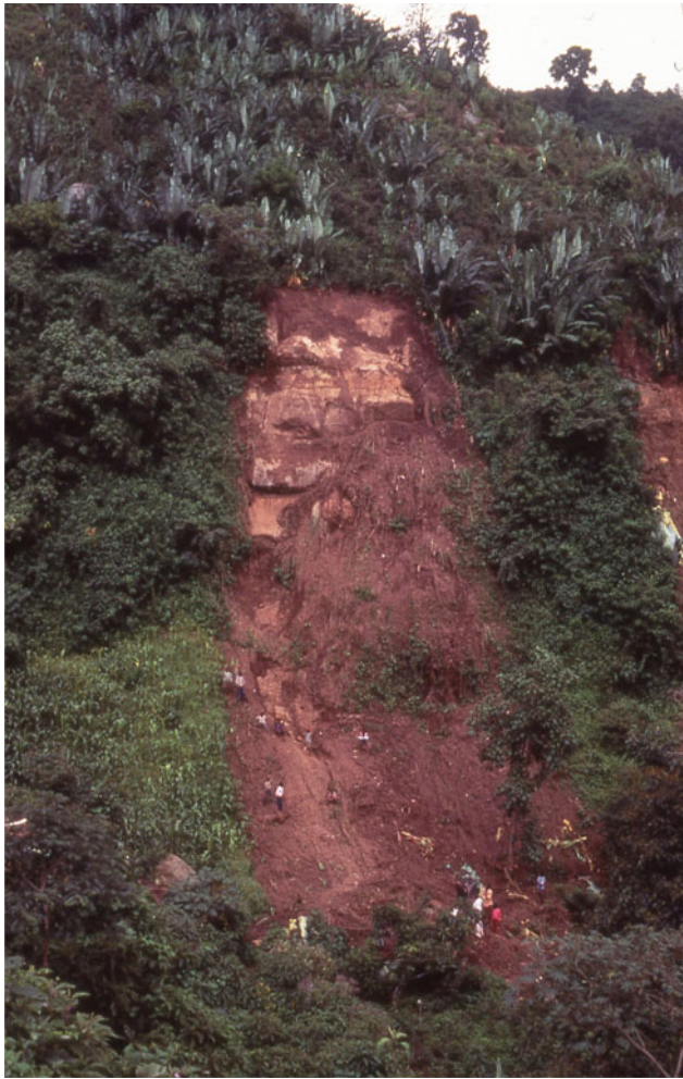
Fig. 20.13 Debris slide at Wendo Genet. Note people climbing the talus for scale
