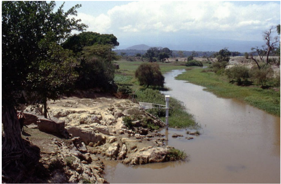
Fig. 4.12 The flow gauge on the Ketar R. near Ogolcho ( 08^{\circ} 01' 58''\text{N} – 39^{\circ} 01' 08''\text{E} ). The streambed is incised into poorly consolidated volcanic ash
