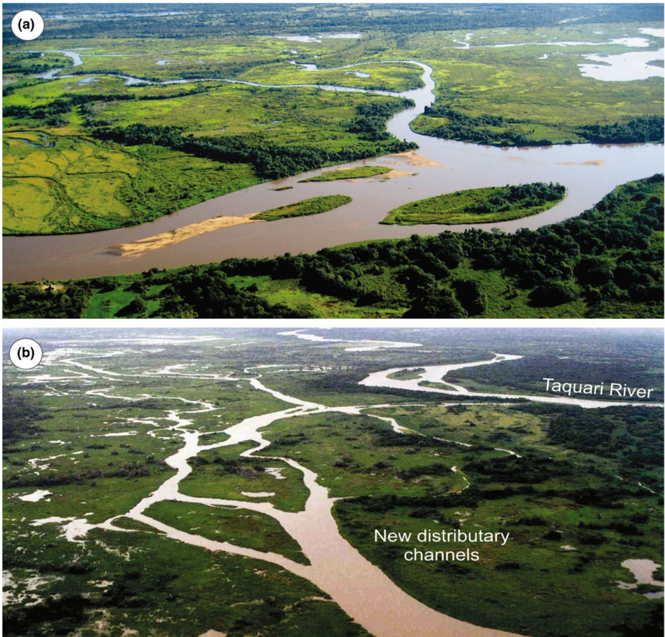
Fig. 12.6 Crevassing of river levees and formation of distributary channels in the right margin of the Taquari River; the avulsion processes are changing the river course (oblique aerial photographs taken in February 2000)
