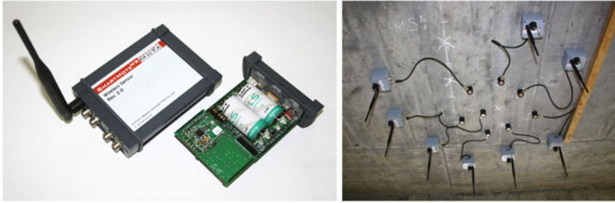
Fig. 2.6 Example of a wireless sensor mote ( www.smartmote.de ) and measurement of acoustic emission and strain data at a concrete structure [10, 11]
