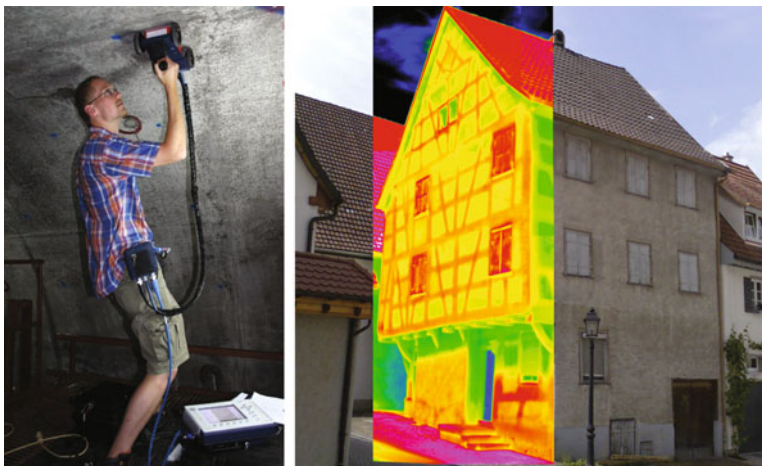
Fig. 2.3 Contact-free NDT applications like Radar ( left ) and IR-Thermography ( right ) enhancing the measurement speed ( right picture by courtesy of Dr. J. Frick)
