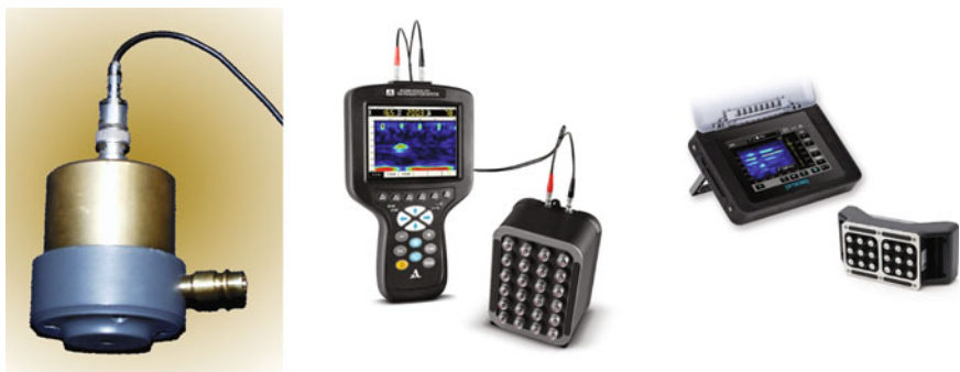
Fig. 2.4 Ultrasound techniques like air-coupled transducers ( left ) or point-contact transducers ( right ) are developed to speed up NDT measurements
